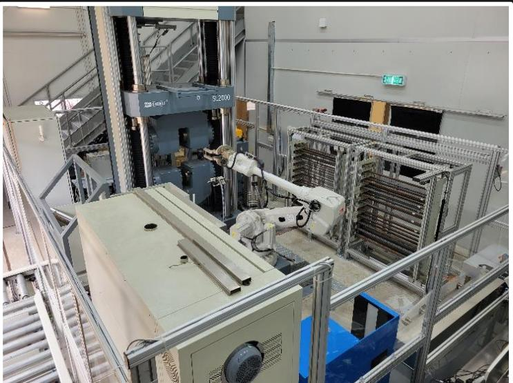
Automated concrete cube testing system
